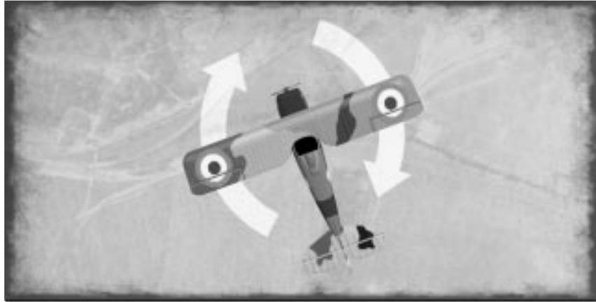
**TO YAW LEFT, APPLY LEFT RUDDER; TO YAW RIGHT, APPLY RIGHT RUDDER.**
