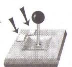
The keypad keys emulate the eight directions of the joystick.
